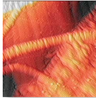
Native Collagen fibrils exhibiting the typical 67nm banding pattern. Scan size 8.5 \mu m.
